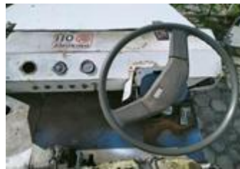
Figure 4. The indicator panel is damaged
