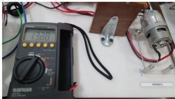
Figure 13 DC Generator Testing
