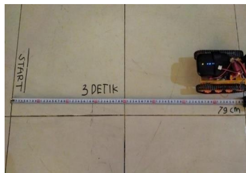
Figure 7. Photos of Testing the Forward and Backward Movement of the Robot
